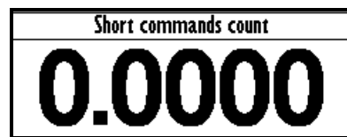
Example of diagnostic value representing the number of illegal control drive sequences
